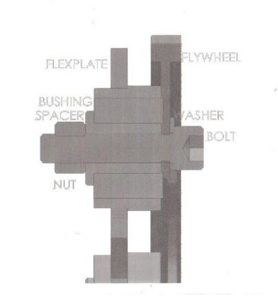
Only sung bolts/nuts at this time. Once all are snug, rotate engine through 3-4 times to allow soft drive to find its own center. Tighten down the (6) bolts/nuts to 45 FT/LBS. If plates are bowed, your flywheel will need to be checked for flatness with a dial indicator. If it is not flat, use a flat pry bar to flex until flat. Reassemble and rotate engine to be sure flywheel and flex plates are flat and parallel. Then retighten bolts to recommended spec.
